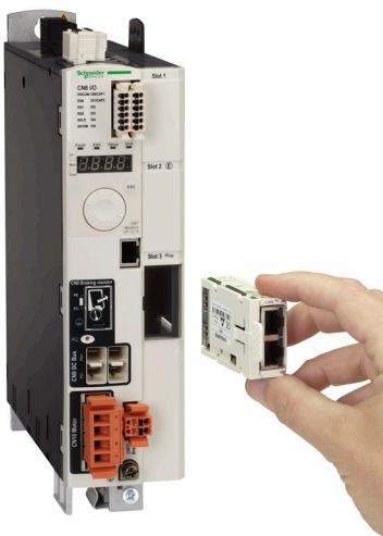
Installing the CANopen communication card VW3A3608
